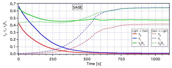
Figure 6: The evolution of the light transmittance  $\tau_v$ , the solar direct transmittance  $\tau_e$ , and the energy load coefficient  $\tau_e/\tau_v$  for the SAGE glass, when switching from bright (1) to dark (2).
