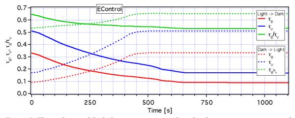
Figure 5: The evolution of the light transmittance  $\tau_v$ , the solar direct transmittance  $\tau_e$ , and the energy load coefficient  $\tau_e/\tau_v$  for the EControl glass, when switching from brightest (1) to darkest (5) transmittance.
