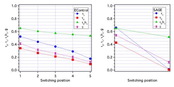
Figure 3: Light transmittance  $\tau_v$ , solar direct transmittance  $\tau_e$ , energy load coefficient  $\tau_e/\tau_v$ , and g-factor for the EControl glass depending on the colouring state. The markers give the values where as the lines are guides for the eyes.
