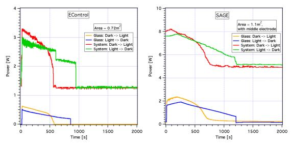
Figure 7: Power consumption of the EControl glass during the switching from the bright (1) state to the darkest (5) state or vice versa and afterwards keeping this status.
